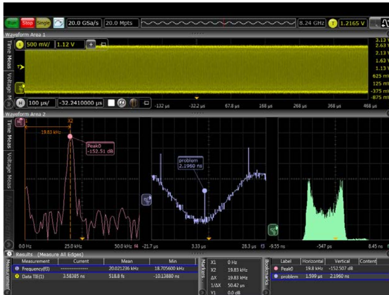
Figure 8. Jitter analysis using a Keysight Infiniium Series oscilloscope with the EZJIT option
