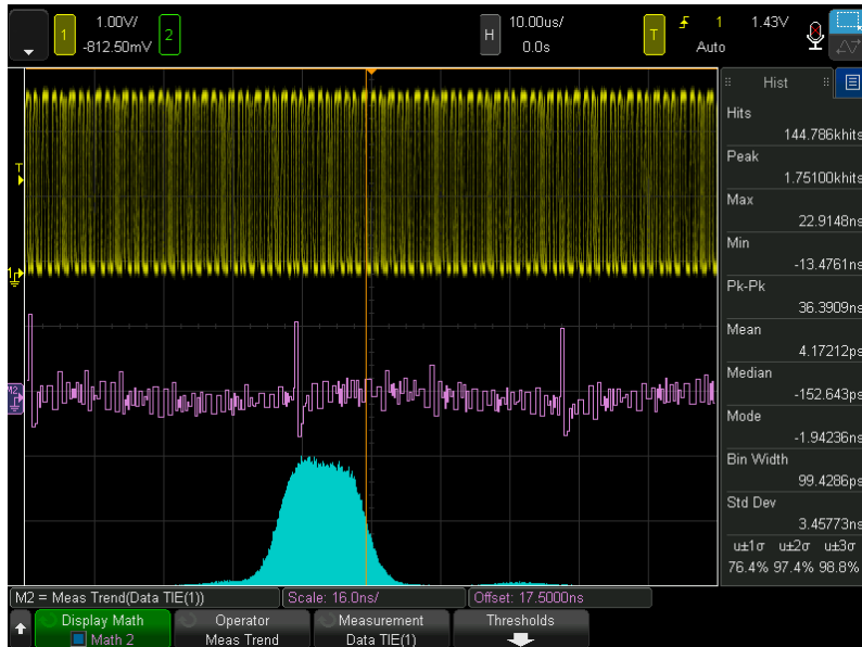
Figure 6. Jitter measurements using a 1st order PLL clock recovery algorithm makes the jitter histogram when compared to figure 4 look less bi-modal and more Gaussian.
