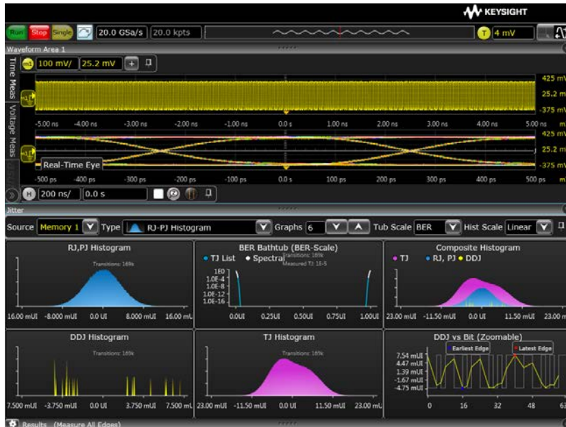
Figure 10. Jitter separation and TJ extrapolation using an Infiniium Series oscilloscope with the EZJIT+ option
