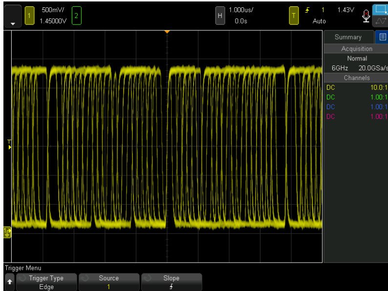
Figure 2. Repetitively capturing a continuous serial bus data signal while triggering on the data signal.
